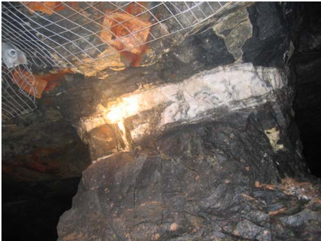
Figure 2: High grade quartz vein present within pillar seen in previously mined airleg stope from Poseidon underground.
